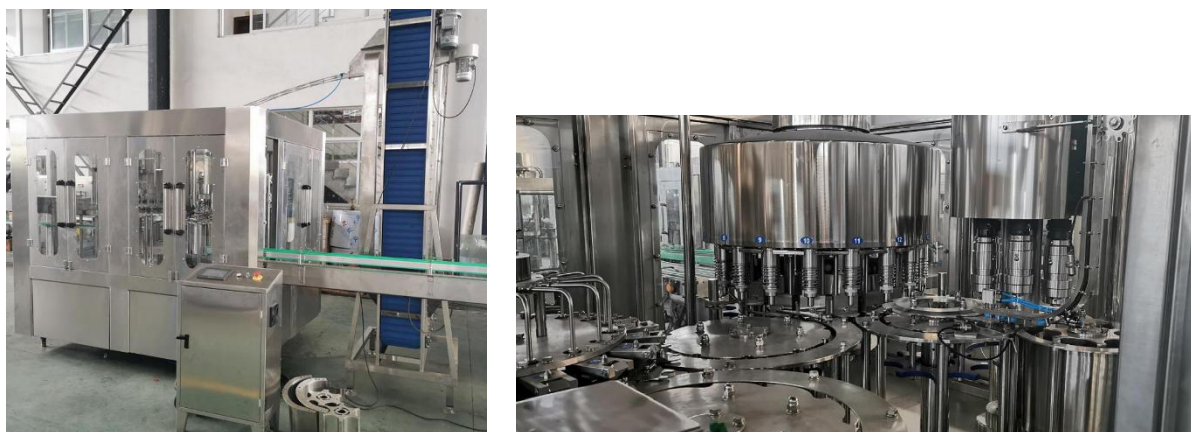
Figure 8.4: 3in 1 High Speed Water Filling Machine
