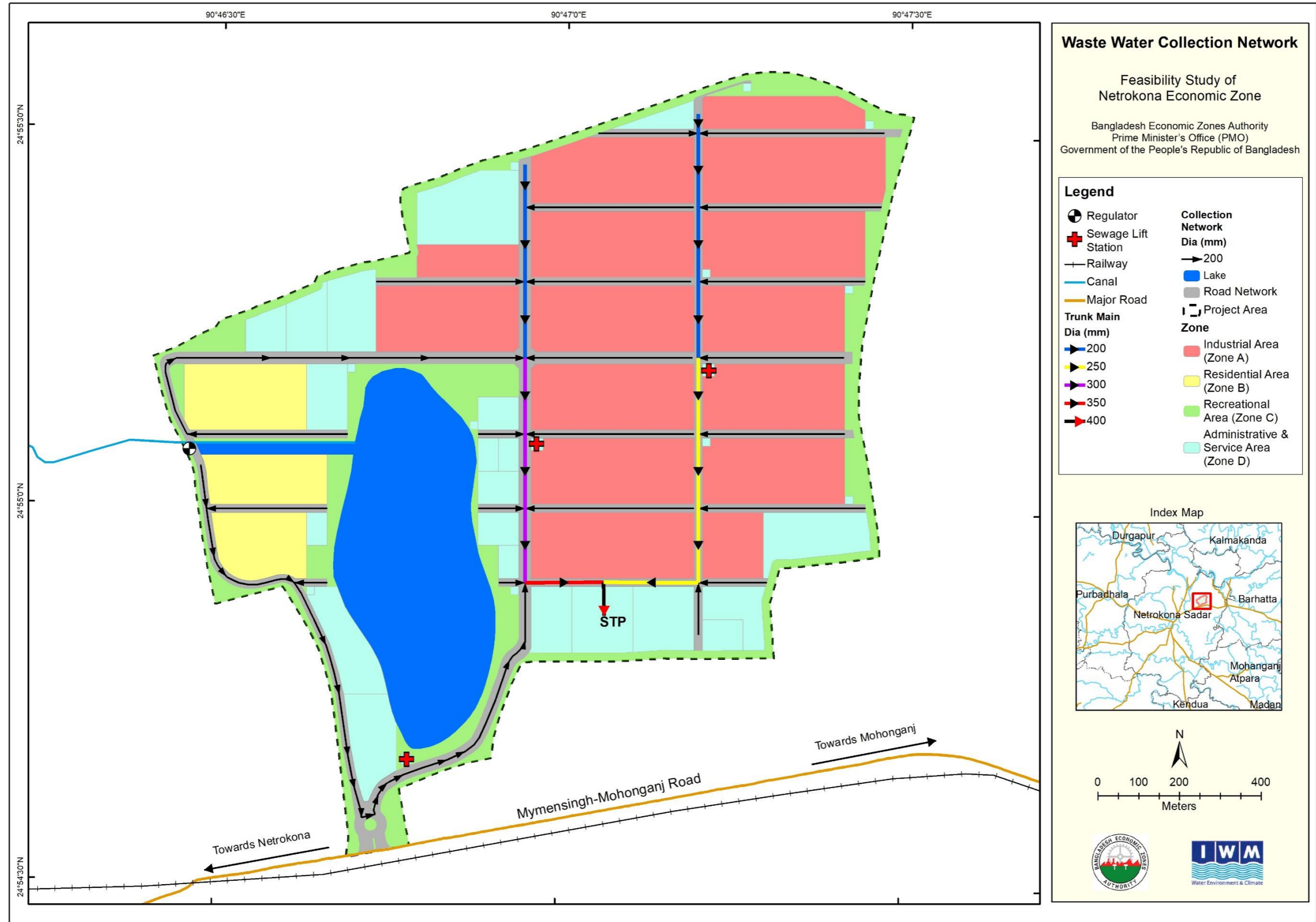
Figure 3: Domestic Wastewater/Sewage Collection Network Map
