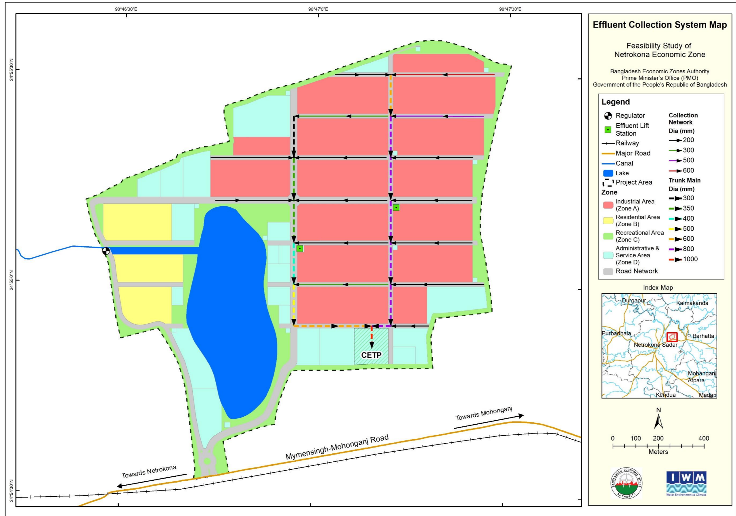
Figure 4: Effluent (Industrial Wastewater) Collection Network Map
