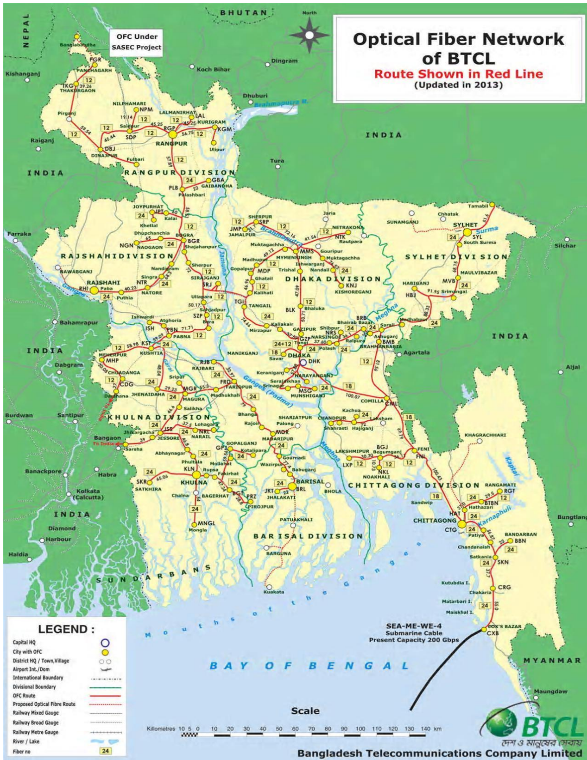
Figure 3.4.1.2-2: BTCL Optical Fibre Links (OFC)
