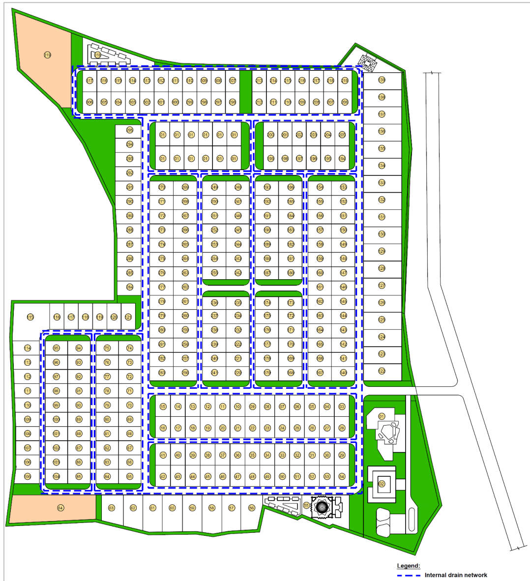
Figure 91: Internal storm water drain network
