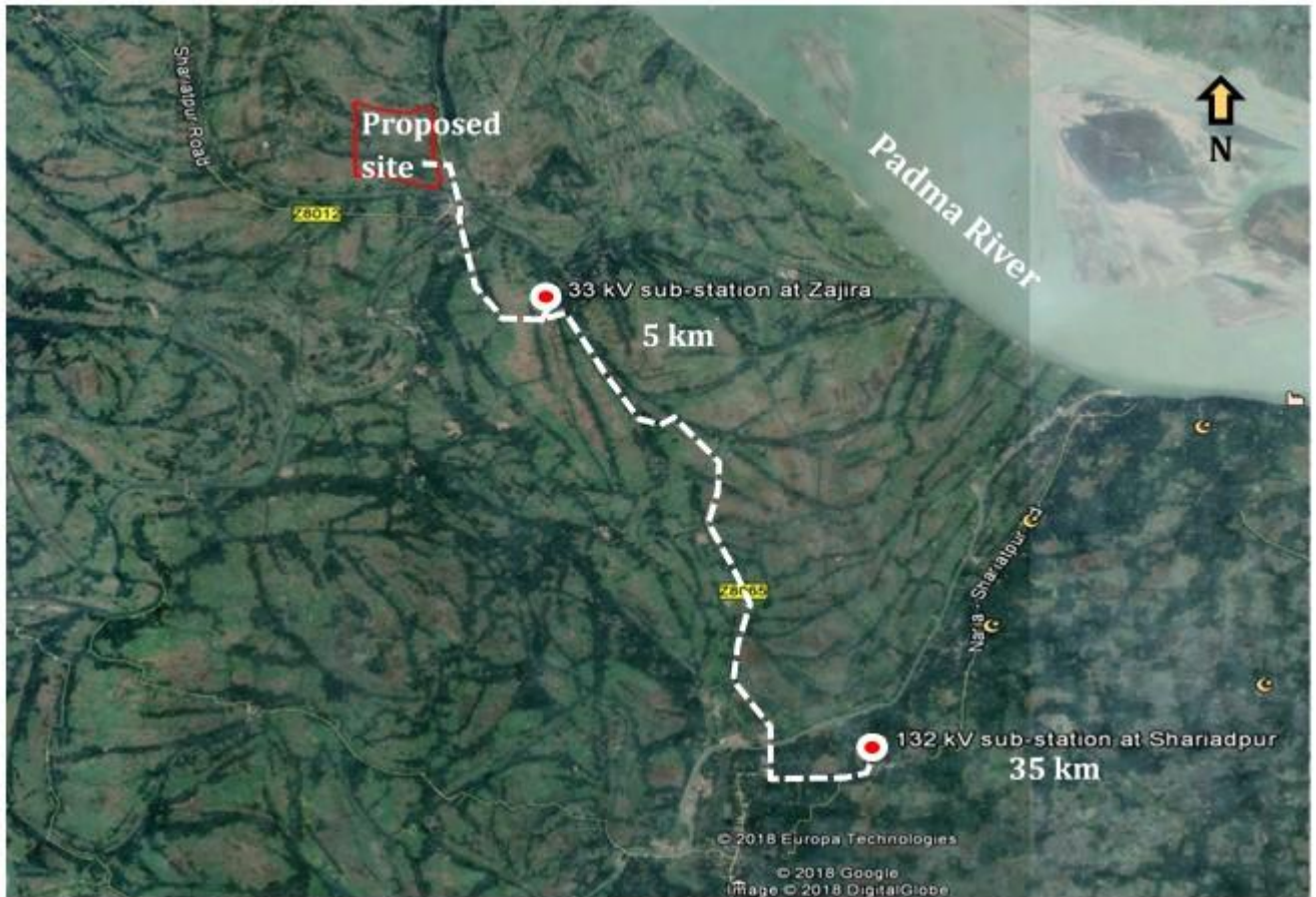
Figure 53: Details of External Power Supply System
