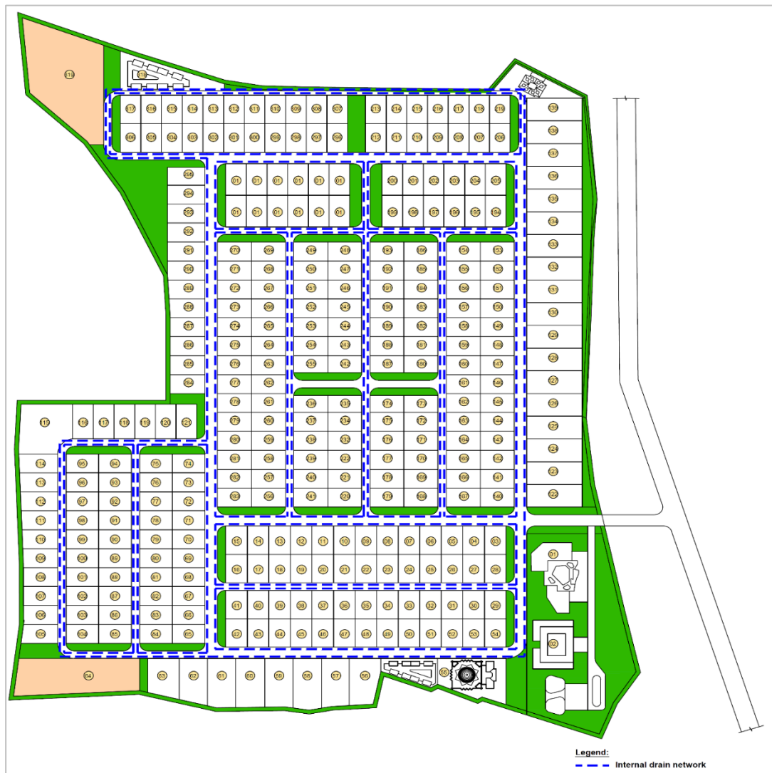
Figure 79: Internal storm water drain network
