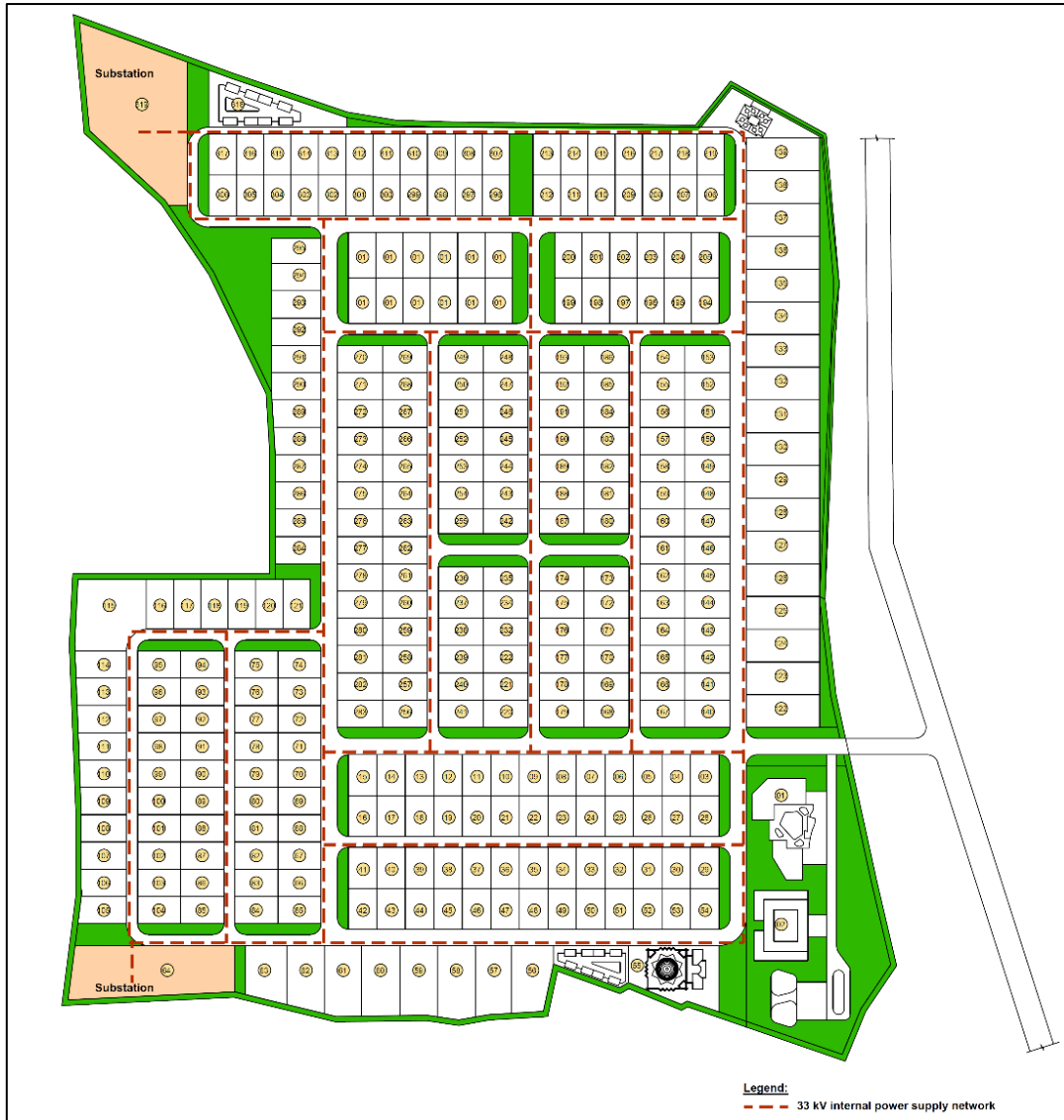
Figure 73: Power supply network inside the EZ
