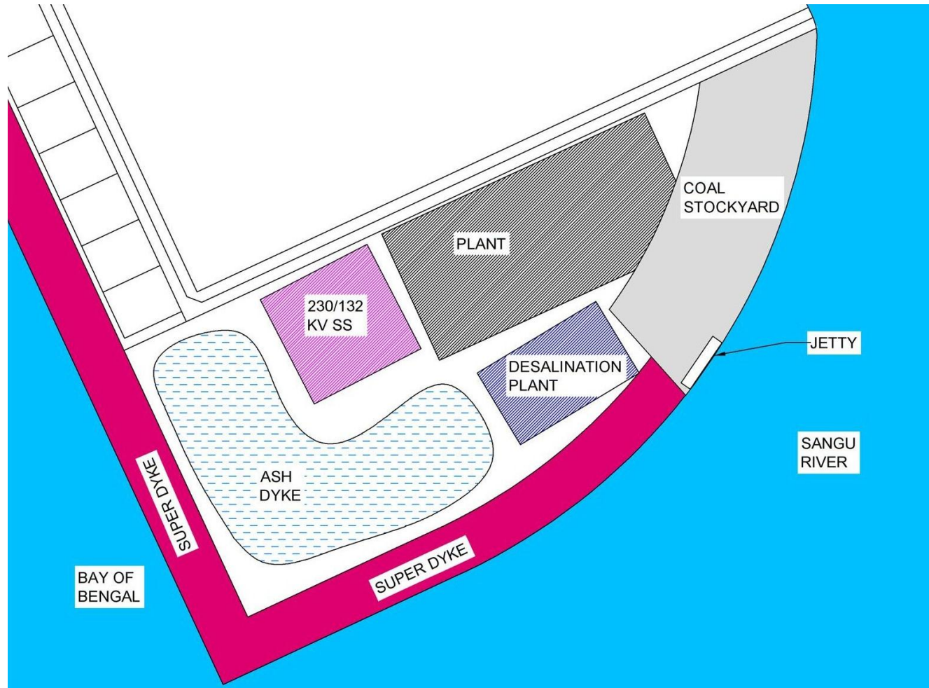
Figure 3.11-3: Typical Layout for Power Plant and Jetty
