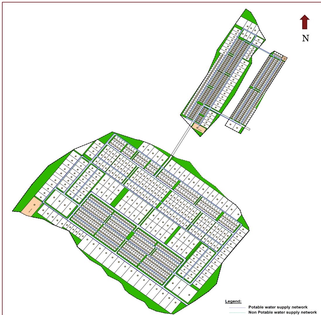
Figure 72: Potable and non-potable water supply network
