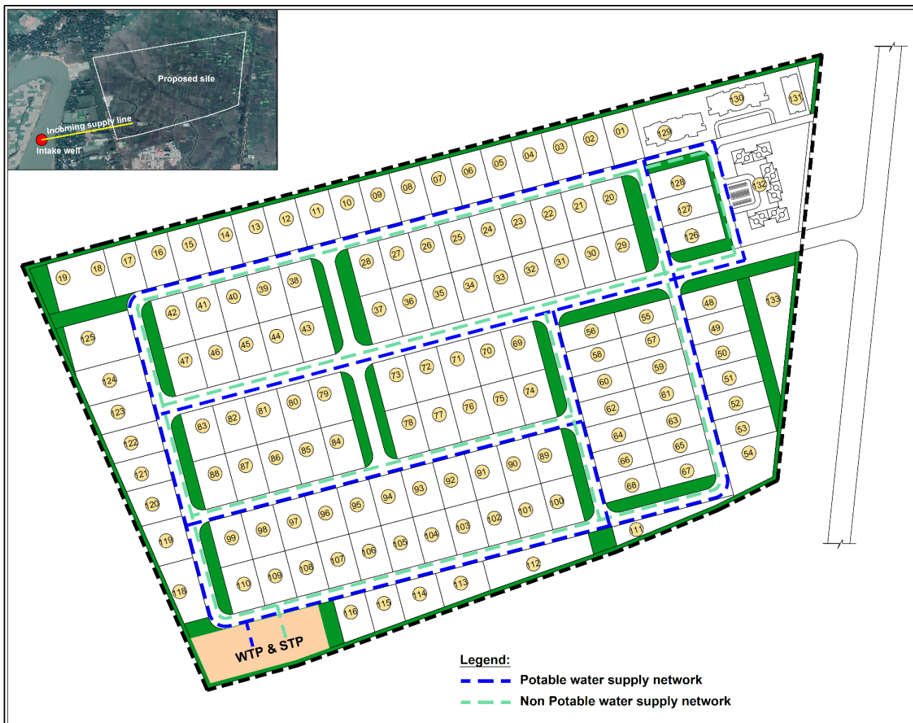
Figure 71: Potable and Non-potable water supply network
