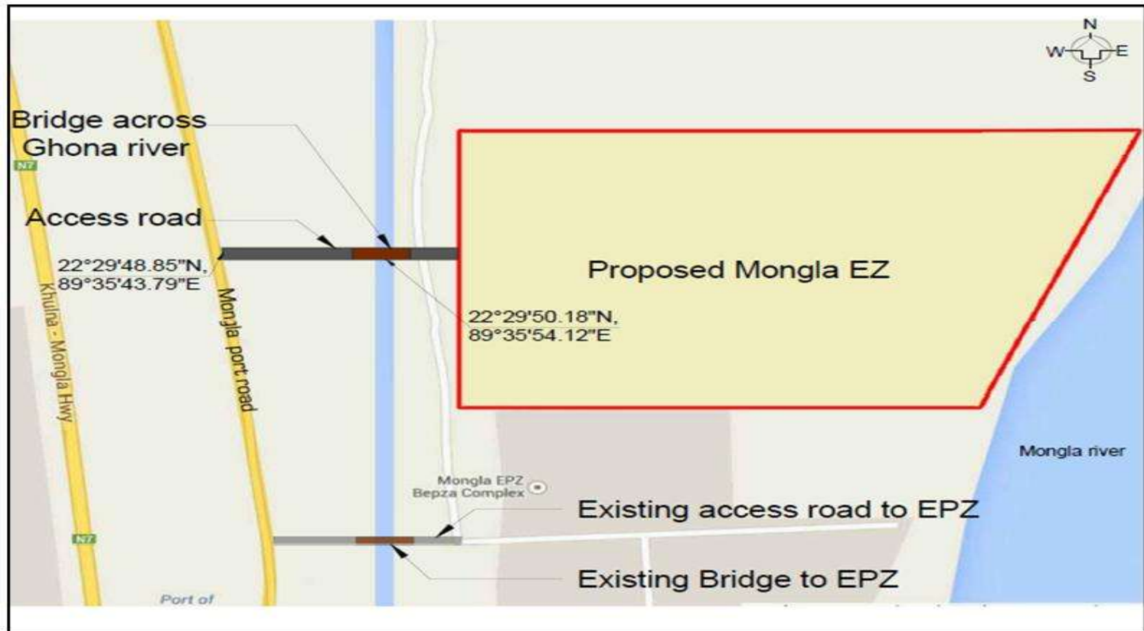
Figure 11: Alignment of access road and bridge
