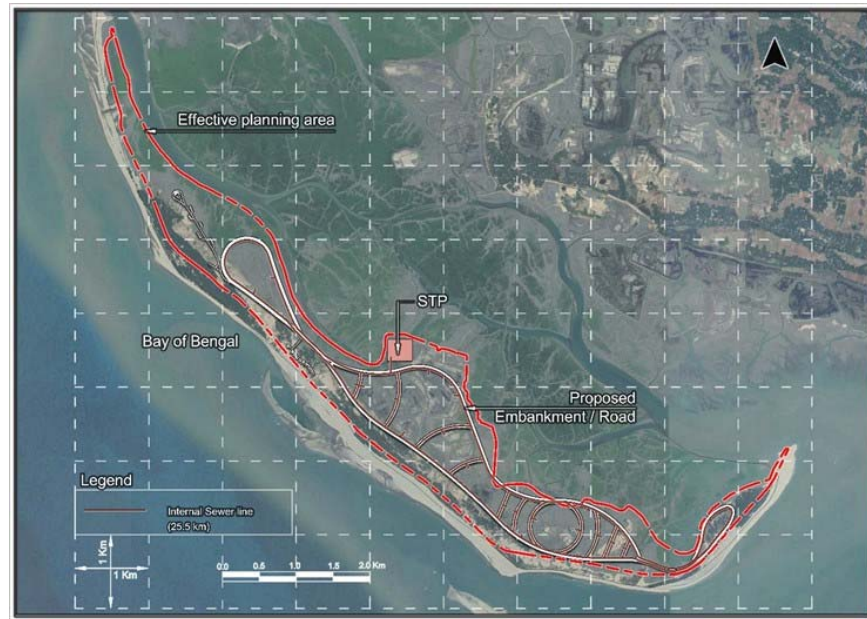
Exhibit No. 12.9: Sewerage network layout
