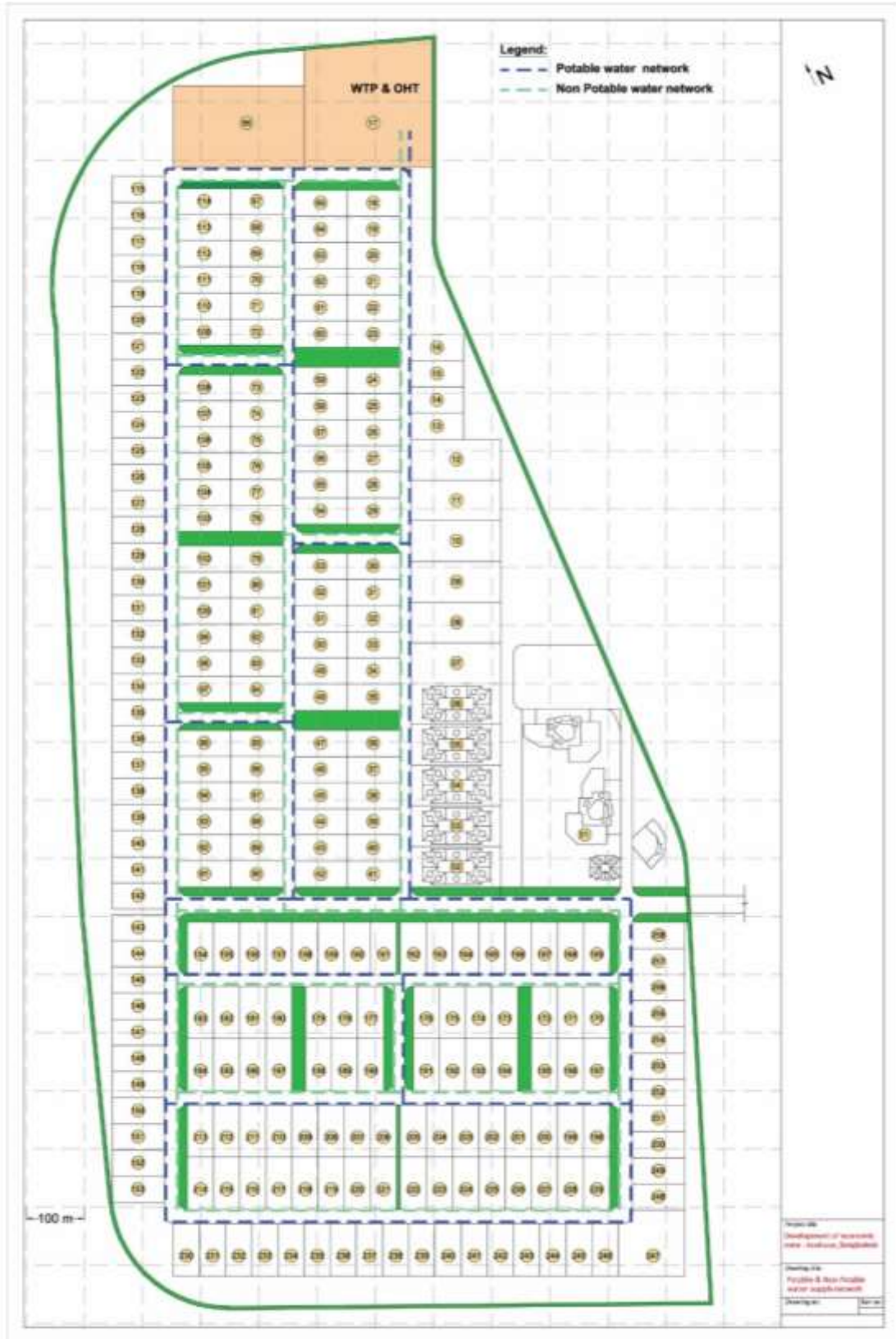
Figure 79: Potable and Non-Potable water supply network
