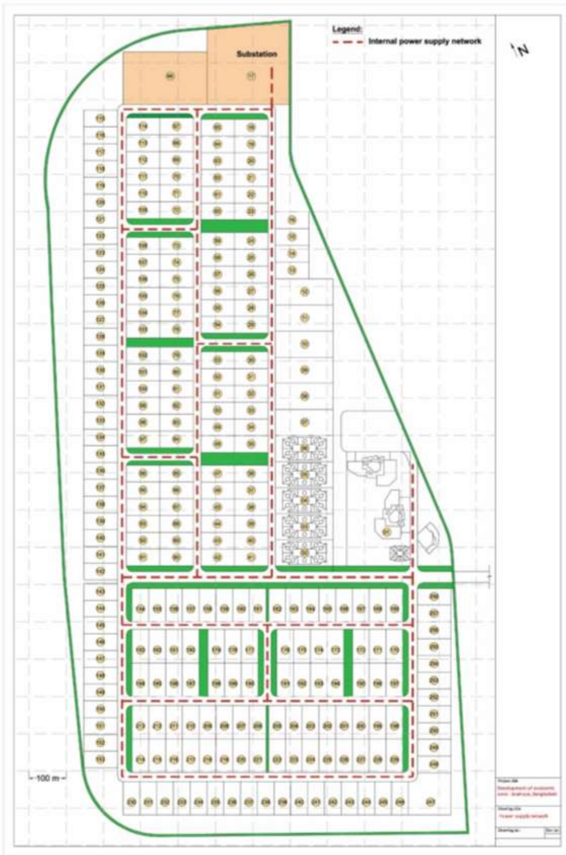
Figure 78: Internal power supply network of EZ
