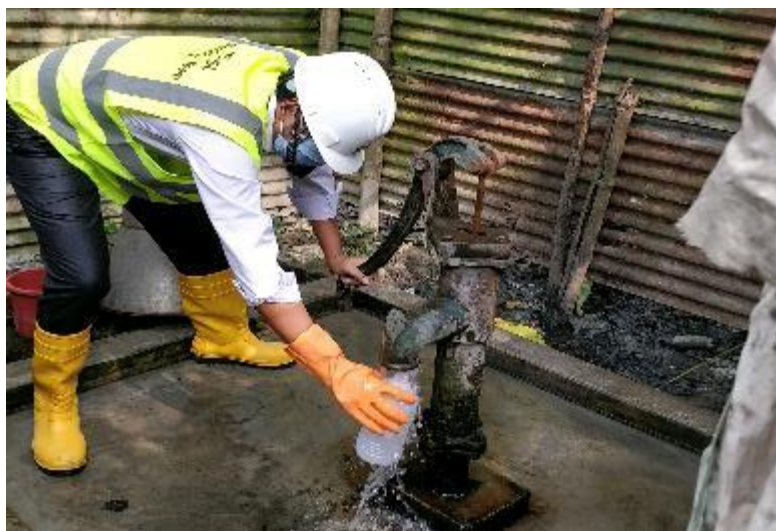
Figure 3.5: Ground Water Sample Collection
