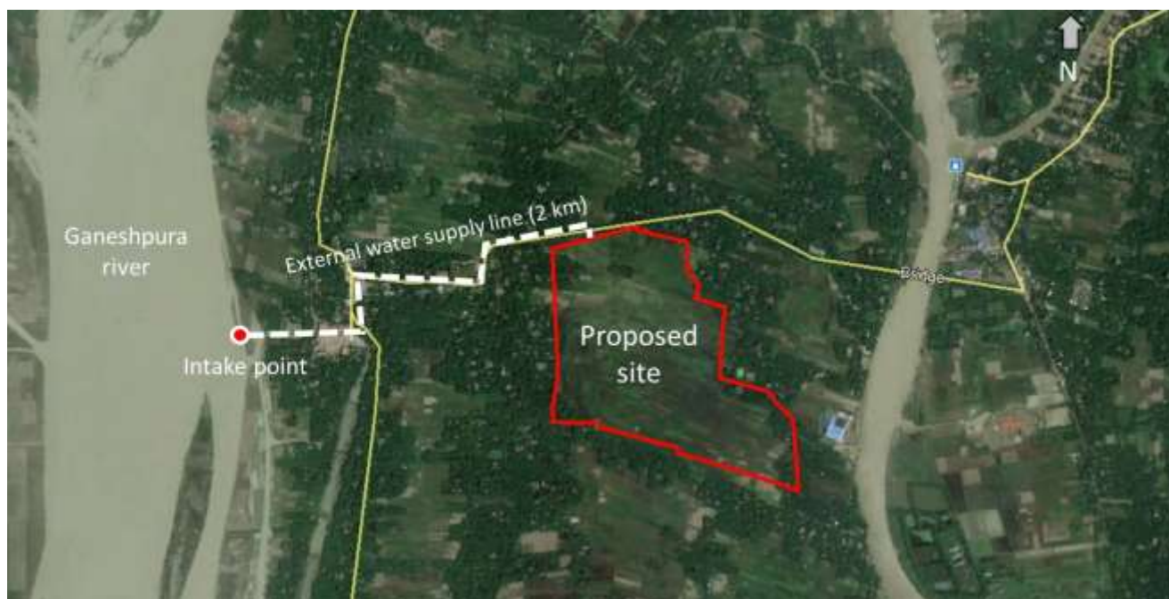
Figure 81: Details of external water supply system
