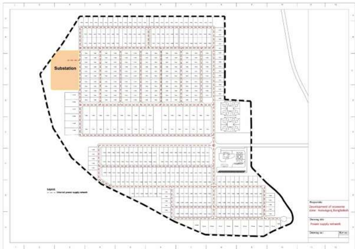
Figure 75: Internal power supply network of EZ
