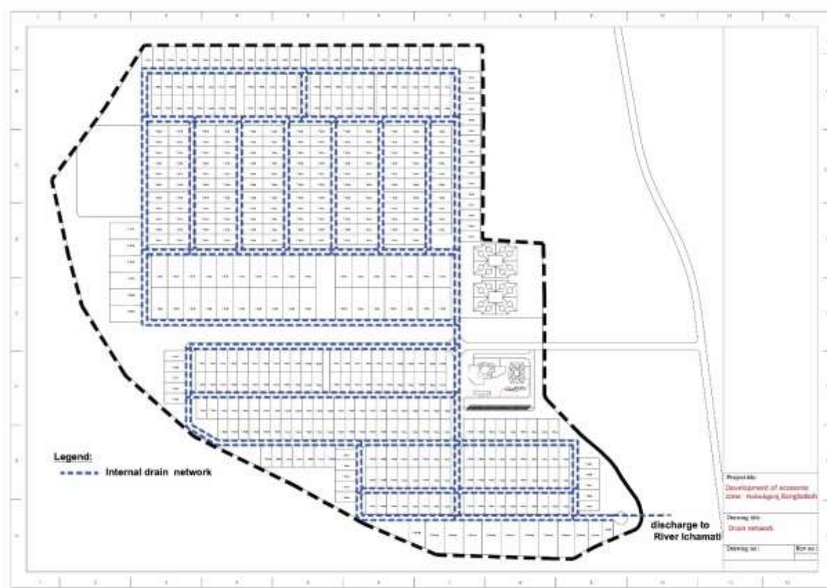
Figure 78: Internal storm water drain network
