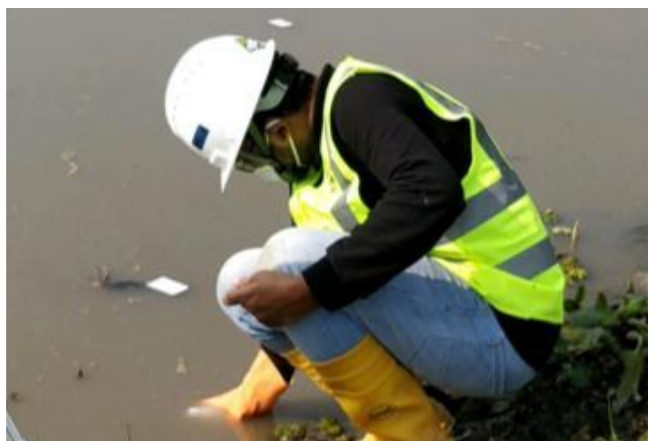
Figure 3.4: Surface Water Sample Collection
