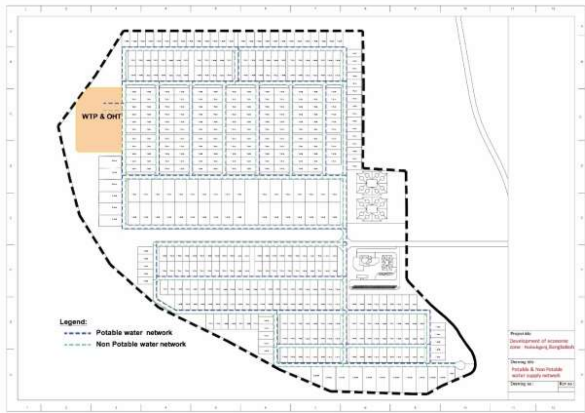
Figure 76: Potable and Non-Potable water supply network
