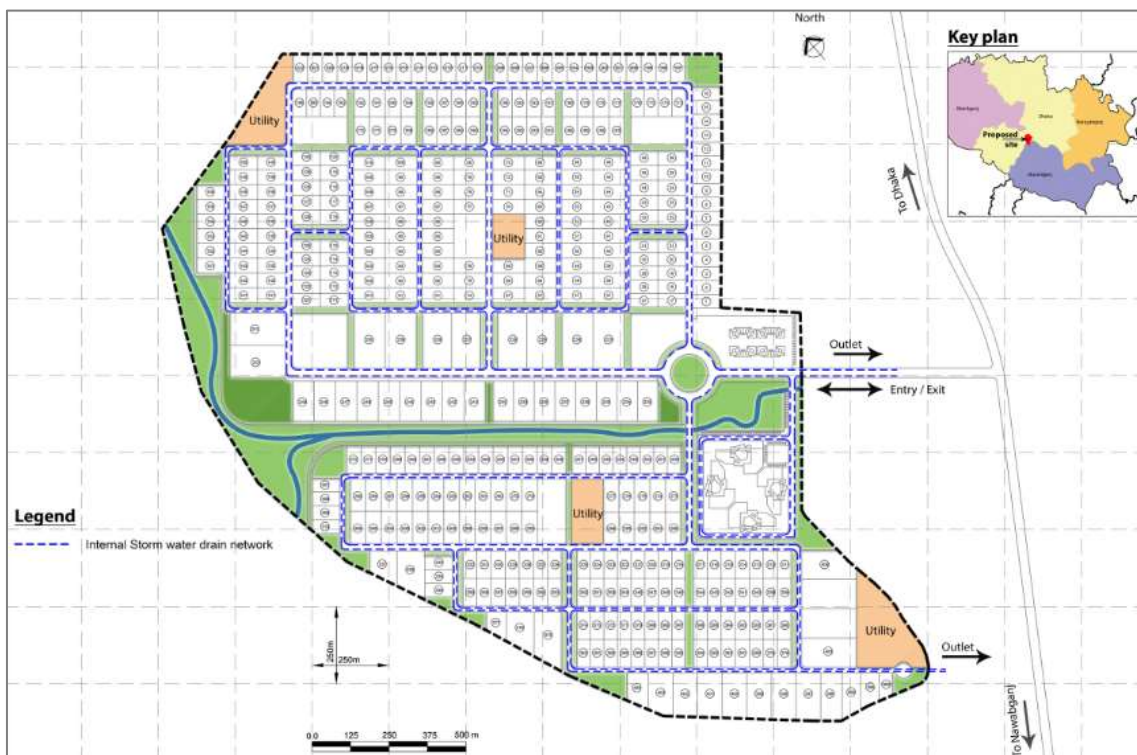
Figure 93: Internal storm water drain network
