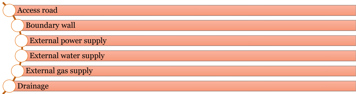
Figure 54: Off-site infrastructure components
