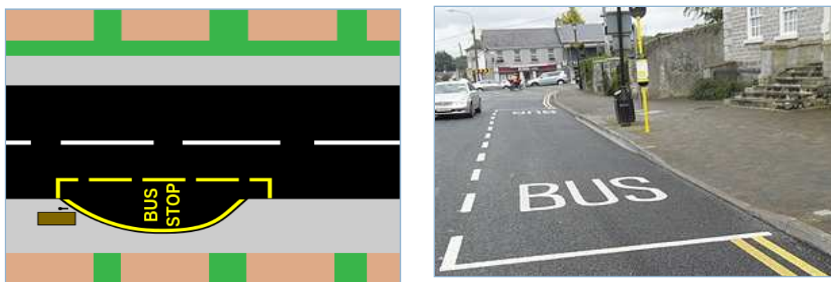
Figure 2-9: Diagram of a Bus Bay and Actual Bus Bays in UK
