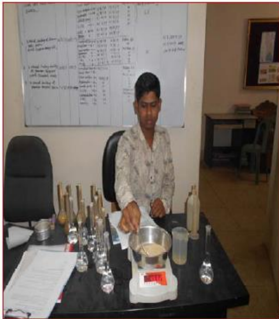
Laboratory test for Specific gravity and Moisture content test
