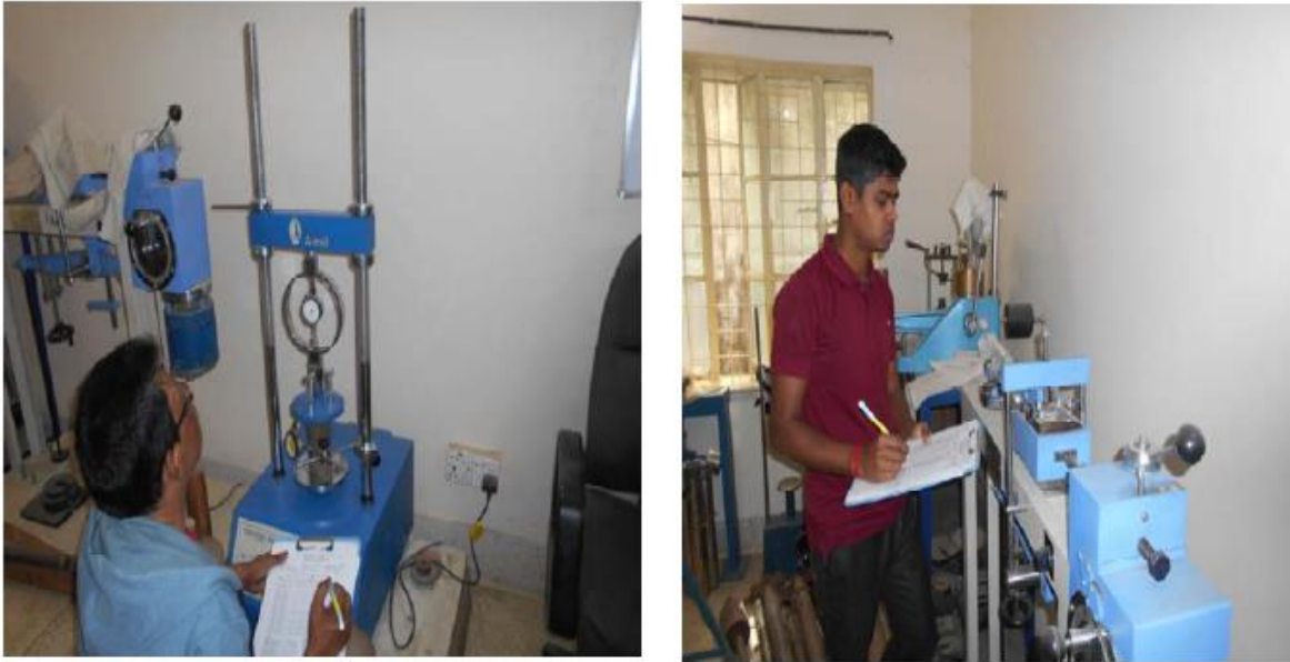
Laboratory test for unconfined compression and Direct shear test.
