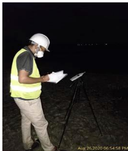
Noise inspection at Night time
