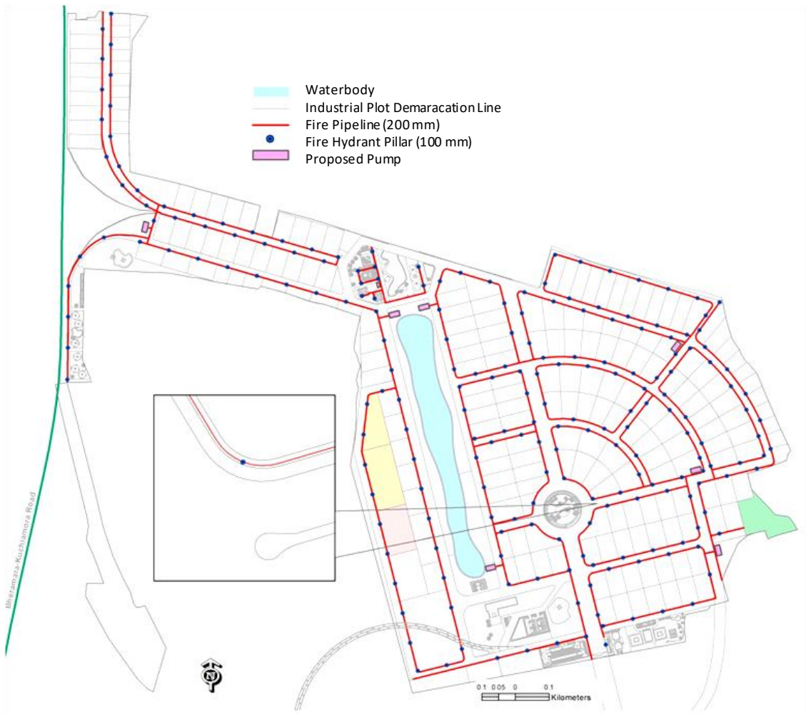
Figure 4.27: Fire Fighting System Network
