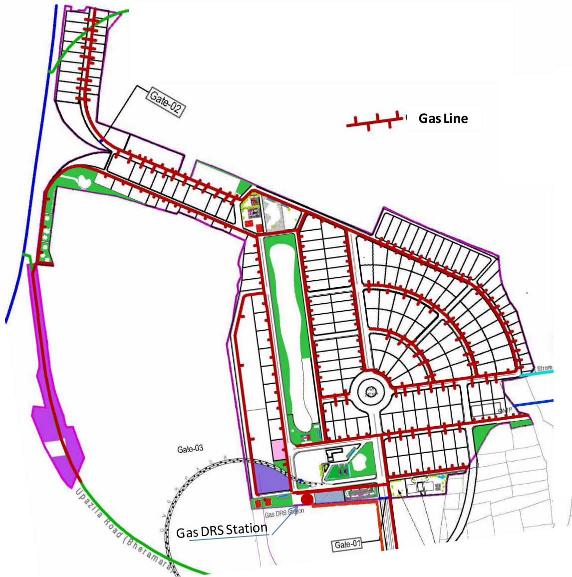
Figure 4.21: Internal Gas Distribution Network
